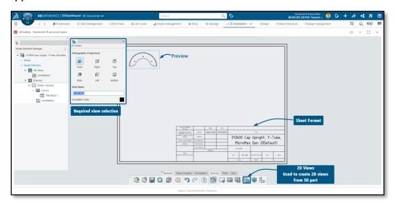
By using this we can create many simple views in the drawing sheet to complete the drafting. Also, the projected views can be added to the sheet using the projected view command:
